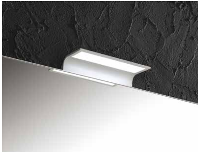
FA334 WAVE lamp, Matt White finish Dimensions: 30x13x5H cm LED 6Watt 12 V with transformer 4000K° / 260 Lumen IP44
